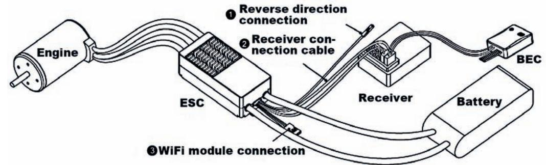
Please make sure that all solder joints are insulated with shrink tubing. The picture shows a reference controller.
