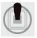
Connect the ESC to the battery, wait 2 seconds, if the motor emits two short „BEEP BEEP“ signals (♪, ♪), the full throttle position is stored.
